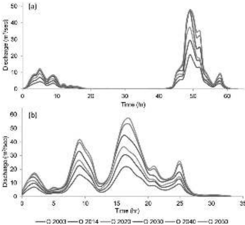
Figure 6. Hydrographs for two frequent rainfall events: (a) December 20–23, 2014; and (b) 11 April 2015. For every rainfall event, the uncoupled WRF-Hydro model was applied using all land-cover maps.
