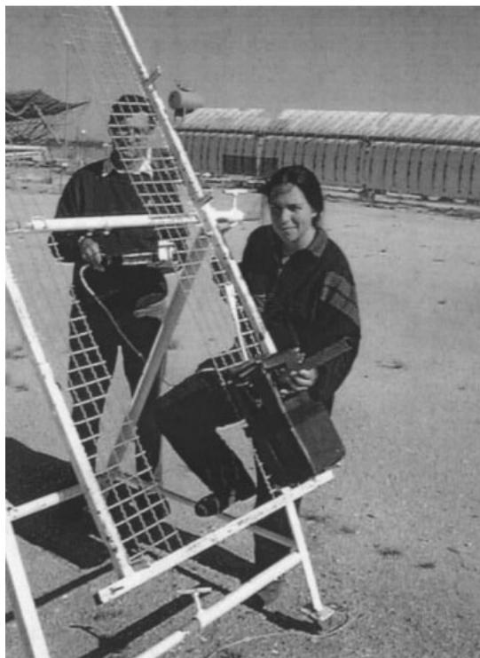
Figure 1. Spectroradiometer strapped to movable stand with collimator tube held in place, the latter is used to find normal incidence, and to remove the sky-diffuse and ground-reflected radiation components
