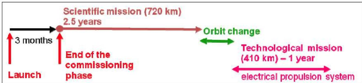
To fulfill its scientific objectives, VEN $\mu$ S will acquire frequent, high resolution, multi-spectral images of over 100 sites of interest all around the world, plus 10 sites for calibration purposes. The satellite will fly in a near polar **sun-synchronous** orbit at 720 km height, 98° inclination. The orbit will be controlled such as to maintain the local time of overpass at +5 minutes.
