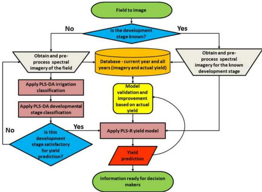
**Fig. 7** Yield prediction analysis steps for a field with either a known or unknown development stage when spectral data are obtained
