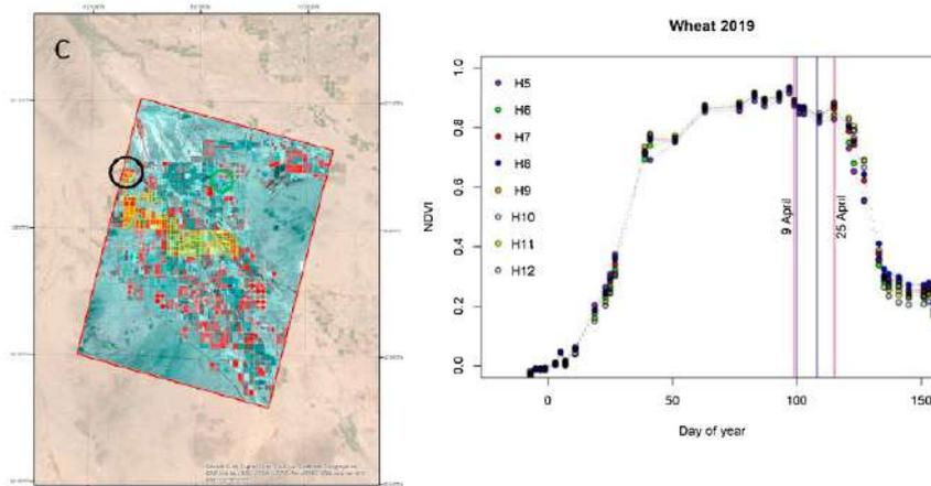
*NDVI time series for 2019 wheat site H8 in Maricopa, Arizona, USA. Atmospherically corrected Venus observations indicated as solid circles. Dotted lines indicate interpolated NDVI. Red vertical lines denote the water stress interval as detected by Venus NDVI. Blue lines denote the onset and end of water stress as based on soil moisture depletion model.*
