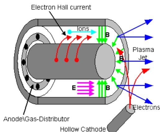
Fig. 1: The principle of an electric thruster
