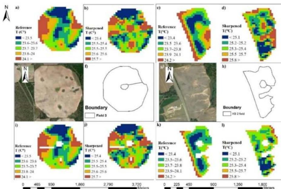
*Field map comparison between reference and sharpened (MODIS/VEN $\mu$ S) maps before and after pixel removal. (a–d) Reference and sharpened maps of the whole area within fields 3 and 9. (e–h) Visual*
