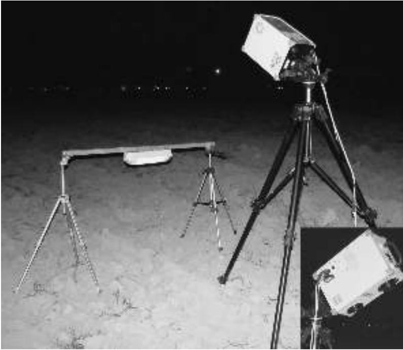
Figure 2. Setup of the 3D Konica–Minolta VIVID910 laser scanner.
