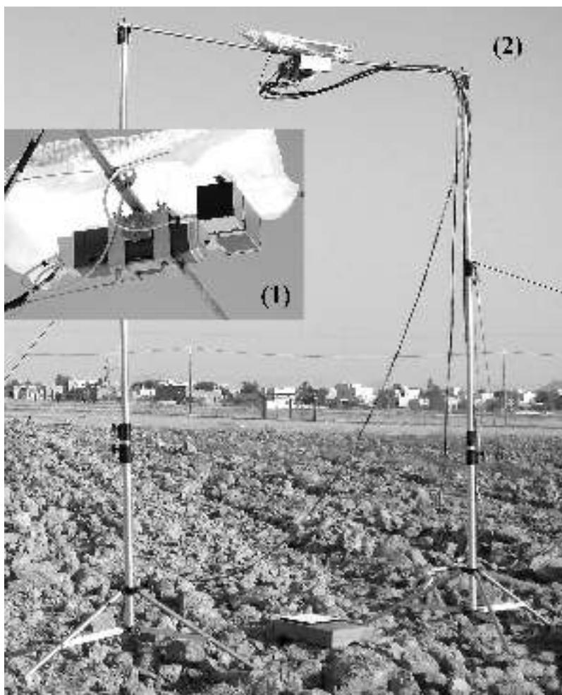
Figure 1. (1) The spectral camera HS; (2) set-up of the camera on a 4 m height construction.
