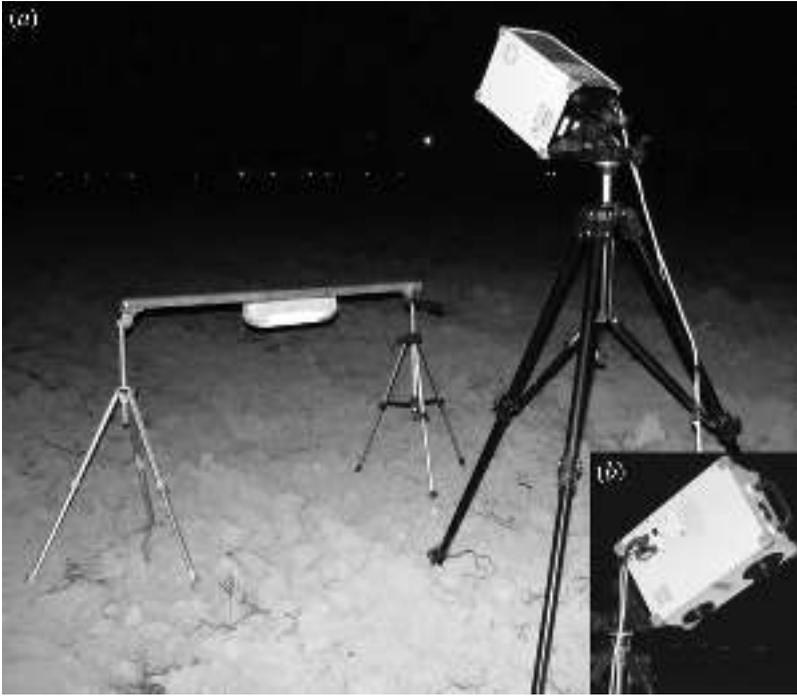
Figure 2. (a) 3D measurement set-up of Konica-Minolta VIVID-910 laser scanner and (b) scanner head.
