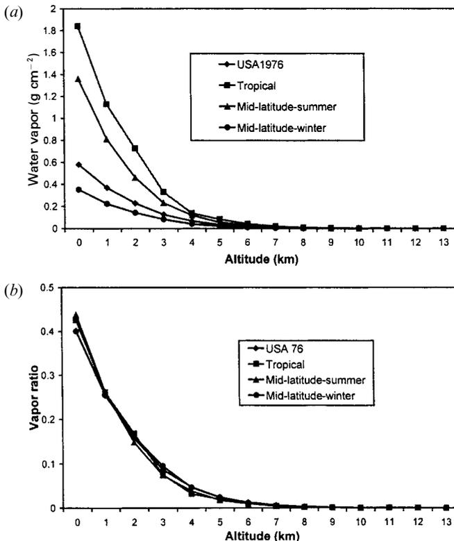
Figure 2. Distribution of water vapour content (a) and its ratio to the total, (b) against the altitude of the profile.
