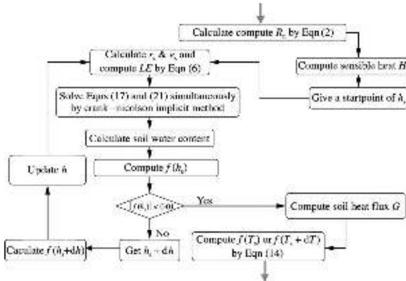
**Figure 4.** The flow chart for computing  $f(T_s)$  and  $f(T_s+dT)$ .
