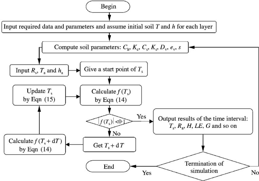
**Figure 3.** The main flow chart of the model's computation.
