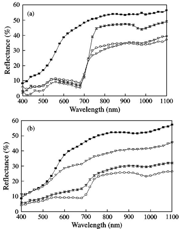
**Figure 2.** Spectral ground measurements of different surface components in the sandy environment during: (a) the rainy season, and (b) the dry season. —■— Sand; —⊗— annuals; —▽— biogenic crust; —□— perennials.
