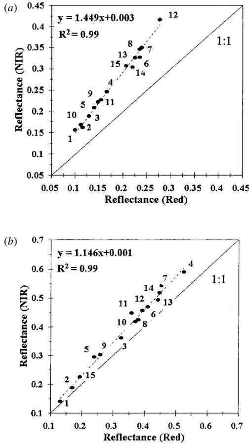
Figure 3. Scatter plots of NIR against red reflectances of the bare surface materials (for key to numbers see table 2) in the study area, showing tendency towards the NIR as the reflectance values increase: (a) Landsat TM data and (b) laboratory spectral measurements.
