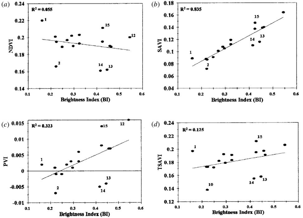
Figure 7. Correlation between vegetation index values and brightness index values of selected bare surface materials; based on Landsat TM data: (a) NDVI, (b) SAVI, (c) PVI and (d) TSAVI.
