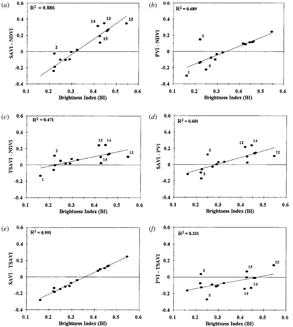
Figure 9. Correlation between brightness and rescaled VI differences ( $\Delta_{VI}$ ) for selected bare surface materials, based on Landsat TM data.
