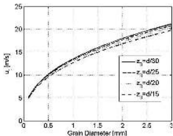
Fig. 4. Threshold velocities at height 3.3 m according to eq 5 as a function of the grain diameter for different choices of  $z_0$ . Parameter values:  $A = 0.1$ ,  $\kappa = 0.4$ ,  $\rho_s = 2710$  kg/m<sup>3</sup> (calcite),  $\rho = 1.2$  kg/m<sup>3</sup>,  $g = 9.8$  m/s<sup>2</sup> (Defoe and Compton, 1925).
