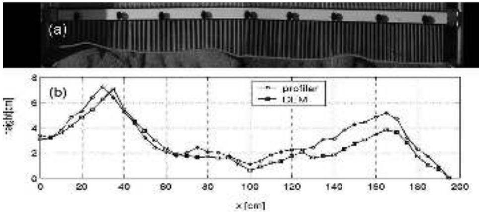
Fig. 6. (a) The profiler used to measure mega-ripple profiles in plot E. (b) The measured and DEM profiles are shown together. (The wind direction is from left to right.) The agreement between the two is highly satisfactory.
