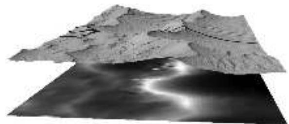
Fig. 5. Two layers that describe one of the plots ( $3.8 \times 2.4$  m). The lower layer is the DEM. White describes the higher elevation places and the dark part, the lower places. The upper layer is the orthophoto of the plot representing it in three dimensions based on the DEM data below it (vertical exaggeration  $\times 2$ ). The orthophoto shows two large mega-ripple crests with small ripples at the trough between them.
