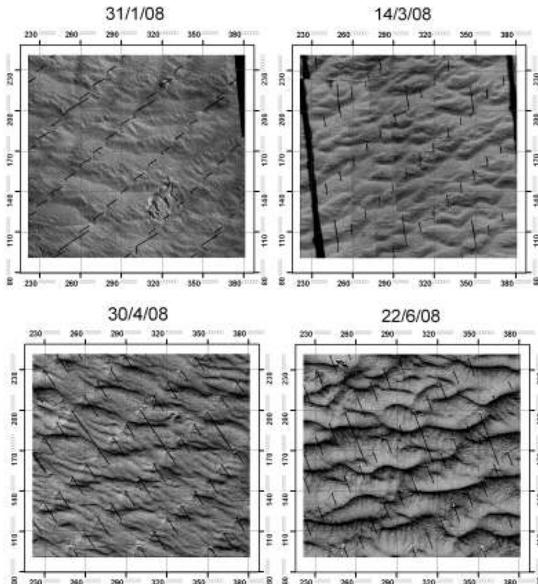
Fig. 12. Ripple evolution from a flat bed (plot A) at four different times, as indicated in the titles, and of a square portion of  $1.6 \times 1.6$  m. The plot was flattened and marked with iron rods in December 2007 (their shadows are seen as black lines). The upward direction in the figure points to an azimuth of  $295^\circ$ . The small ripples coarsened during this period and their wavelength increased to 30 cm. See text for details.
