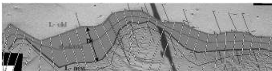
Fig. 4. Schematic illustration of the method used to analyze average ripple movement between two successive measurement times. For this example, the normal to the crests defined as d_i in Eq. 5 was 20.58 cm.
