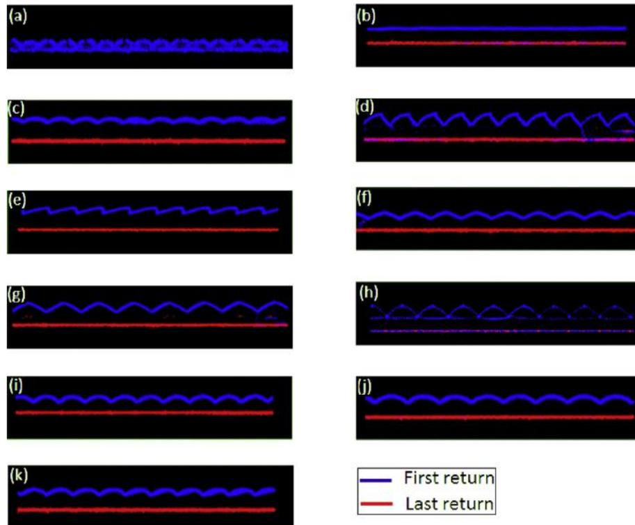
Fig. 7 – Profiles of the LiDAR-derived first and last returns along with the different PA structures (a) Low plastic tunnel; (b) Net-house; (c) Circular net-house; (d) Porched cut edge shape; (e) Saw-tooth structure; (f) Arched shape; (g) Edge arched shape; (h) Net stretched under arched shape; (i) Circular arched shape; (j) Circular wide arched shape; (k) Circular arched shape with 90° rotation.
