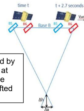
Fig. 2. Illustration of the stereoscopic capability provided by the VEN $\mu$ S satellite. By collecting two images that look at the same scene but at a different angle a Digital Surface Model can be calculated ( $\Delta h$ ) through correlation of shifted ( $\Delta x$ ) around tie-points.
