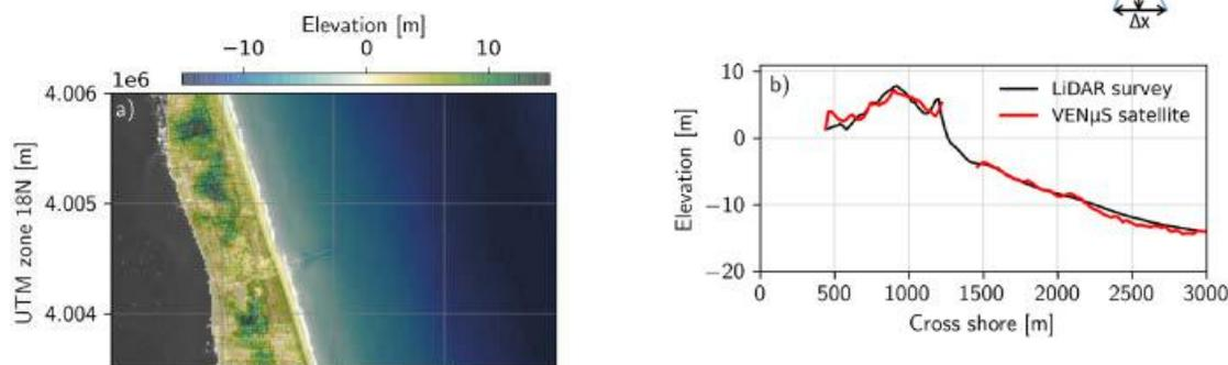
Fig. 3. Spaceborne coastal continuum. a) presents the airborne LiDAR measurements covering land and sea in the vicinity of the FRF at Duck overlaid on top of a Venus image. b) shows the alongshore average profile of the LiDAR survey in black and superimposed the VEN $\mu$ S derived topography and bathymetry in red.
